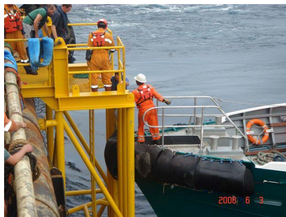
Figure 1 – Personnel transfer from a crew boat to a larger vessel using a 'surfer' (photo: Saipem)
