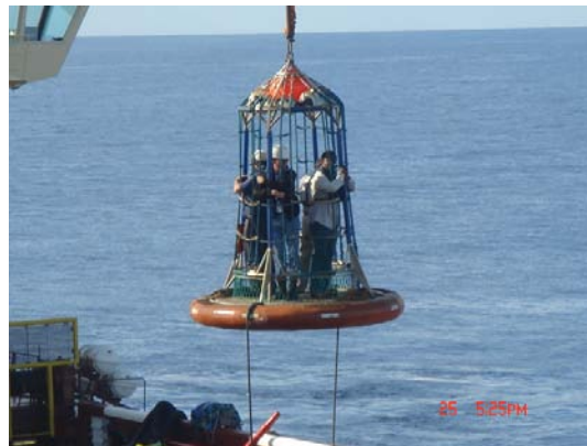
Figure 3 – Personnel transfer using an 'Esvagt' device (photo: Saipem)
