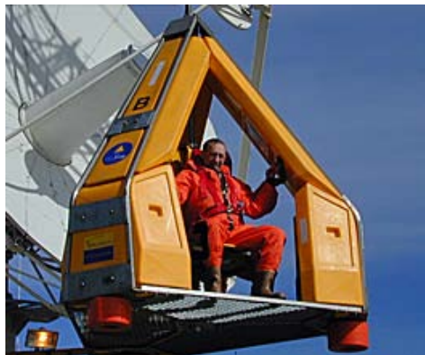
Figure 4 – Personnel transfer using a personnel transfer capsule (photo: Saipem)
