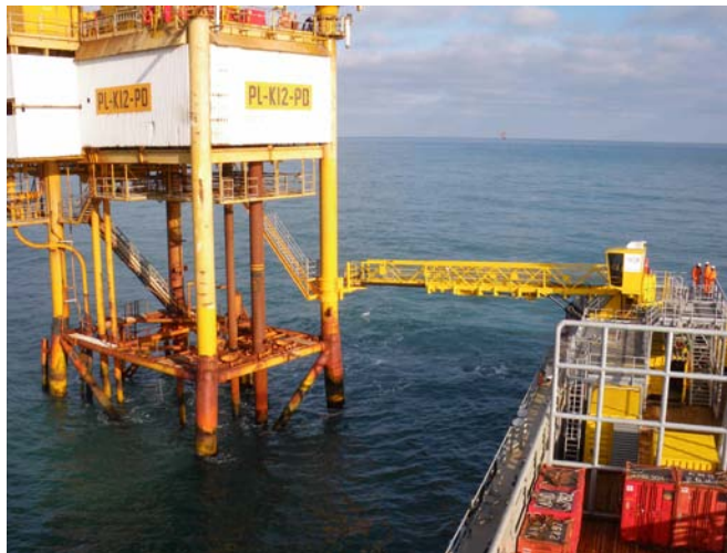
Figure 5 – Personnel transfer using a purpose-designed hydraulic gangway (photo: Mermaid Offshore)
